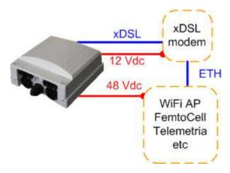
The RPW (power card of DataPowerBoost) can connect a modem and a data collector/distributor device. These units can be housed in the same box or can be installed in close boxes like DPs or cabinets.
